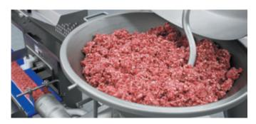
The Handtmann system solution for economic minced-meat production with outstanding quality: VF 600 vacuum filler, GD 93-6 grinding attachment connected to GD 93-3 inline grinding system and the GMD 99-2 minced-meat portioner. For the manufacture of minced-meat products up to a width of 220 mm. The perfect interplay of the processes of grinding and portioning in conjunction with the tray feeding automation option for maximum production standard.
