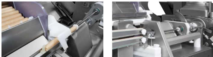
↑ Sausage casing magazine with automatic slug casing spooling
