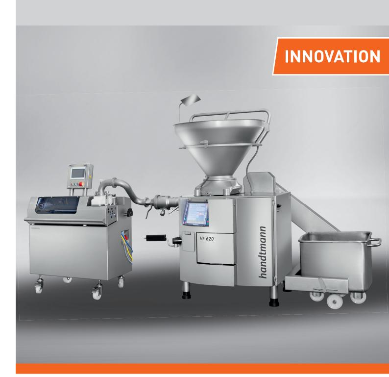
Automatic forming of a variety of products, such as burgers, balls, slices and sticks, with the modular MBF forming system. Round, square or longish – a multitude of shapes in variable product sizes is possible.
