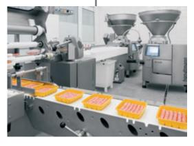
The process steps of collating and depositing are the continuation to the complete solution. Using the Handtmann collating module, portions can be collated in different ways. The precise depositing on the collating belt or the exact depositing in trays are the perfect basis for further downstream automation such as packaging.
