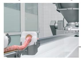
The filling of a continuous sausage rope ensures maximum productivity with superior product quality. The VegaCasing hardens in the fixation solution while the sausage rope is being fed to the conveyor belts of the AL system.
