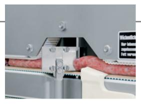
The continuous sausage rope is precisely cut into defined units. The forming process step (ends are formed into sausage-typical round shape) provides an excellent and appetising product for the highest customer demands.
