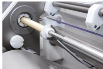
↑ Casing spooling with semi-automatic casing change function
